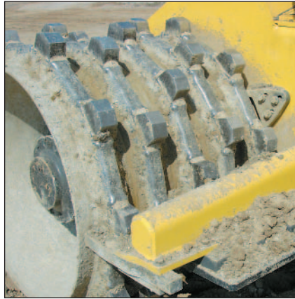
Soil compacting wheel.
