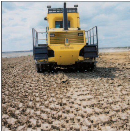
Optimum compaction of large areas with the special BOMAG wheel design.
