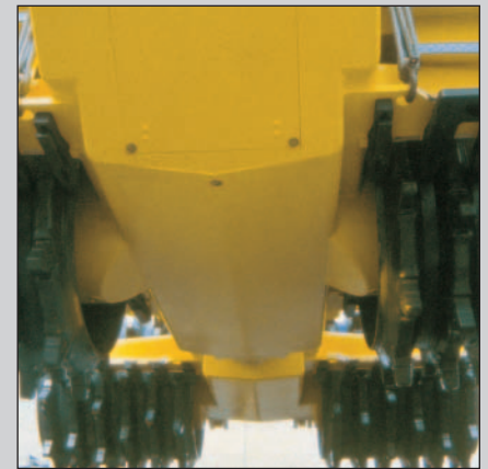
The totally enclosed frame protects all drive components.
