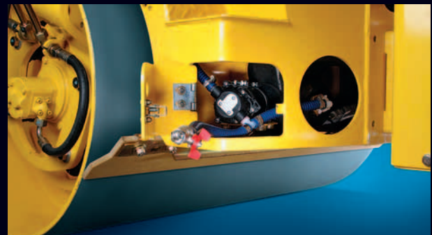
Quick access – water pump and drain tap.
