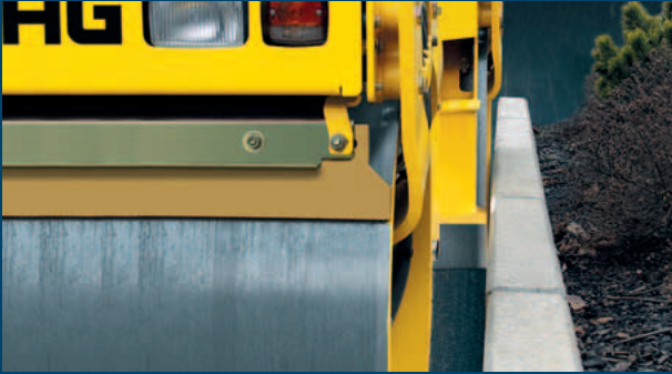
The crab-walk feature gives 4 cm drum offset to either side.
