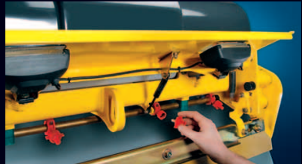
Faster sprinkler nozzle replacement.
