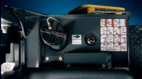
The water level gauge is always visible to the operator.
