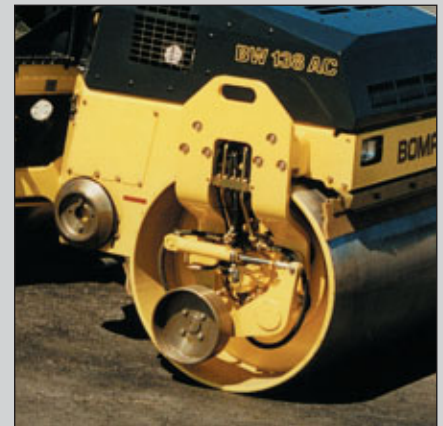
Edge cutter with three tools for cutting and compacting asphalt (option).
