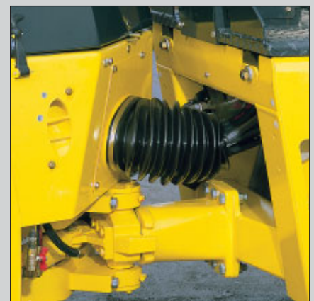
Articulated/oscillating centre joint for excellent manoeuvrability.
