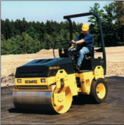
All-round safety for the driver thanks to ROPS bar, safety belt, and seat contact switch.
