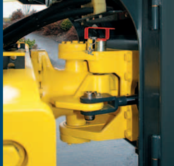
Maintenance-free oscillating articulated joint.
