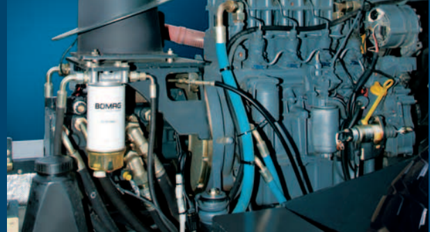
Fuel consumption is reduced with BOMAG ECOMODE technology for DH/PDH single drum rollers. This is an intelligent drive management system based on load-dependent engine speed.
