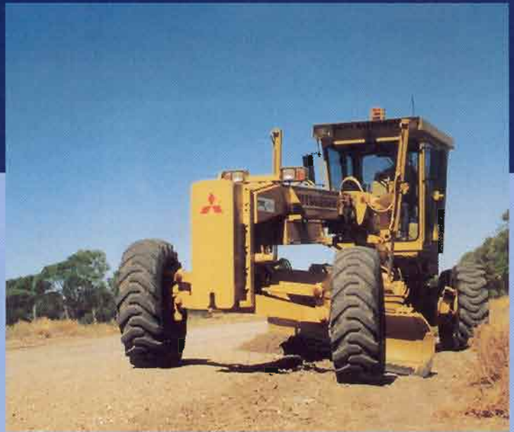
Frame articulates to a maximum 26 deg for crab steering when grading culverts, unstable surfaces and steep slopes.
