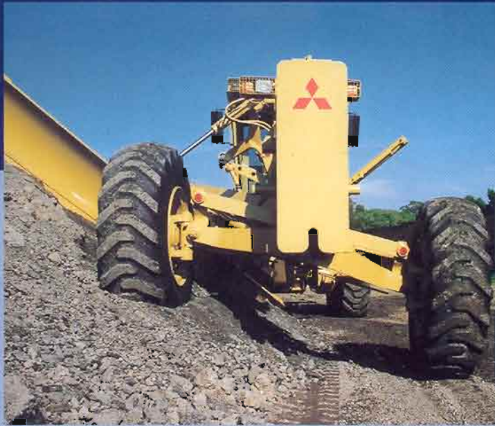
Front axle oscillation for maximum traction regardless of work site conditions.
