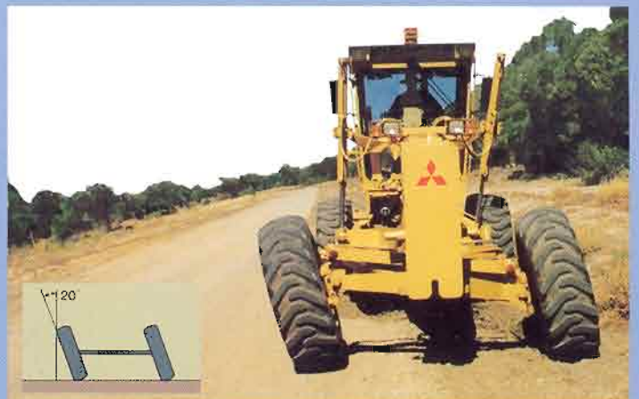
20 degree wheel lean lets the operator control side draft when working with heavy loads.
